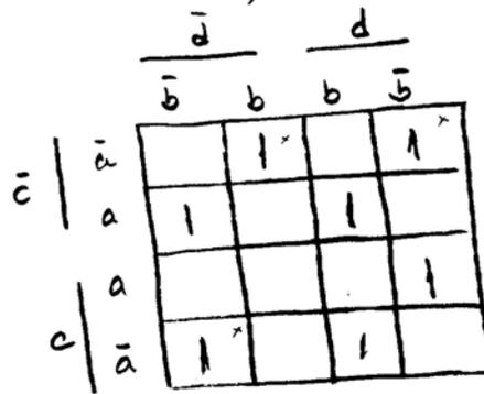
3 bits  $\Rightarrow f(b,c,d) = \bar{b}\bar{c}d + \bar{b}c\bar{d} + b\bar{c}\bar{d} + bcd$
